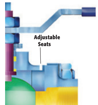
PBM valves seal on the upstream seat unlike conventional floating ball valves.
