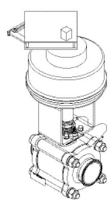
Sanitary Fire Rated Valve with manual fail safe spring return unit
